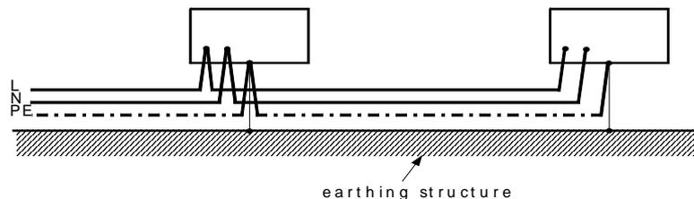
Figure 27 - Earthing arrangement
