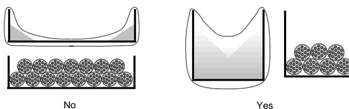
**Figure 10 - Cable arrangement in a metallic section**
