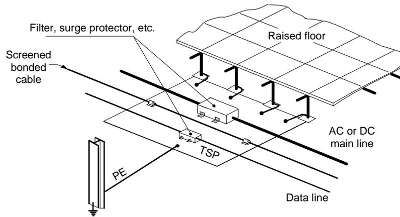
Figure 22 - Example of transient suppressing plate installation details
