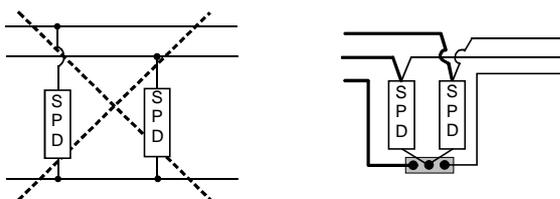
Figure 30 – Short connections of surge protective devices
