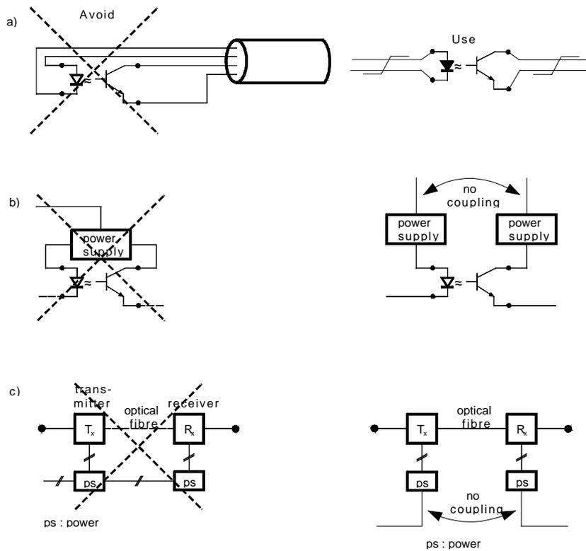
**Figure 29 - Installation guidelines for optocouplers**
