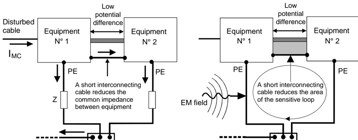
**Figure 16 - Example of low common impedance and small loop**
