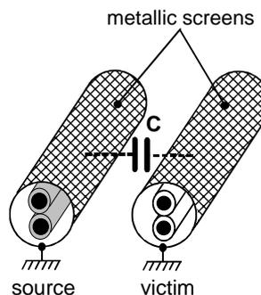
**Figure A.1 - Screened cables reduce capacitive coupling**
