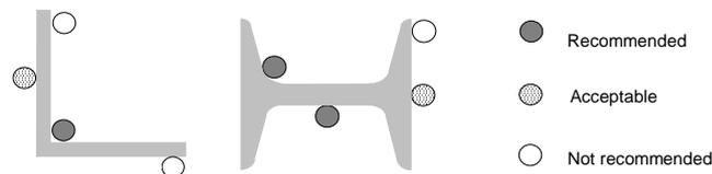
**Figure 12 - Location of cables inside metallic construction elements**
