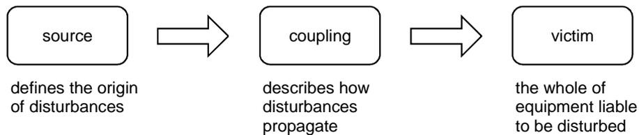
**Figure 4 - Schematic representation of an EMC problem**
