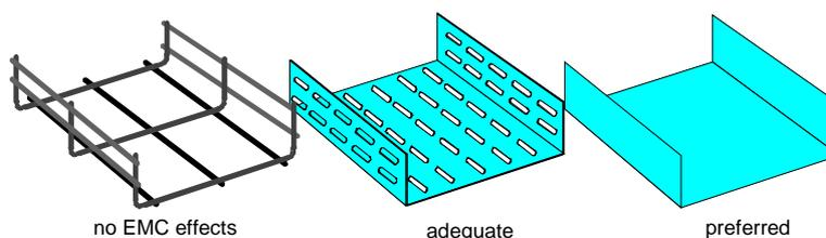
**Figure 9 - EMC ranking for different metallic trays**
