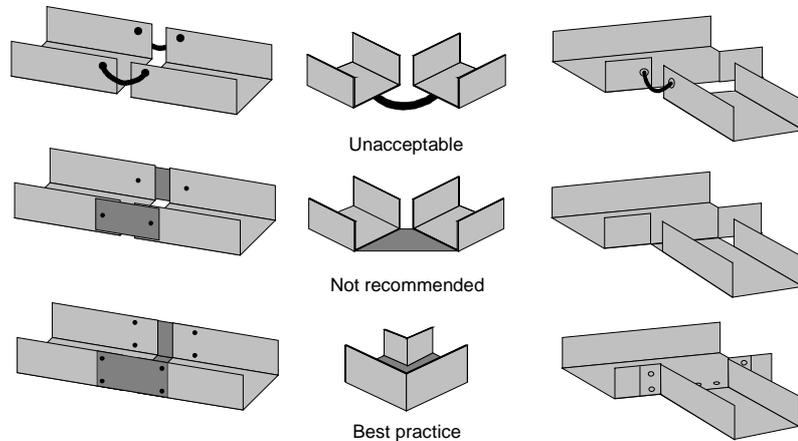
**Figure 11 - Continuity of metallic system components**
