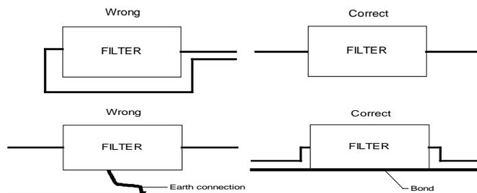
Figure 23 - Earthing and bonding of filters
