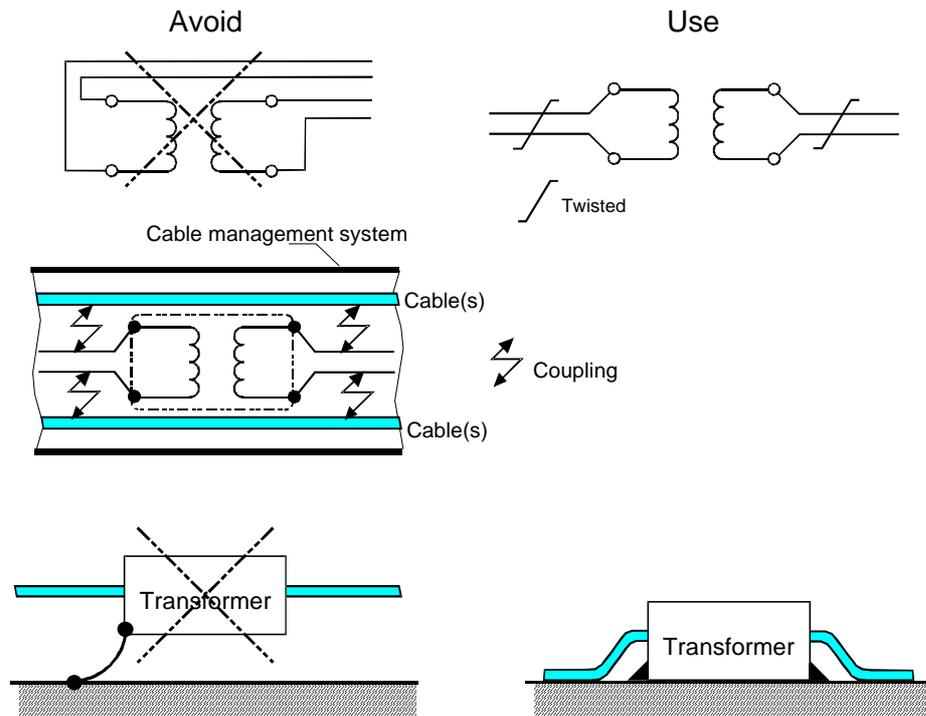
**Figure 28 - Installation guidelines for transformers**
