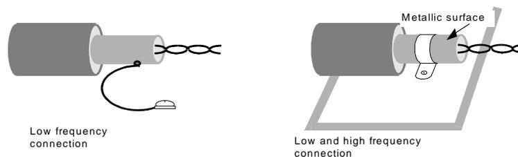
NOTE When a screen or earth conductor exists outside the cable construction it is regarded as a PEC, which should be earthed at both ends. Inner screens or earth leads are also earthed at one or both ends. For TN-C or TN-C-S systems see A.6.2.2.
