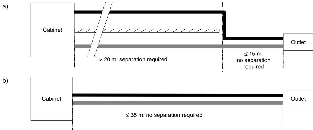
**Figure 5 - Separation between power and data cables**
